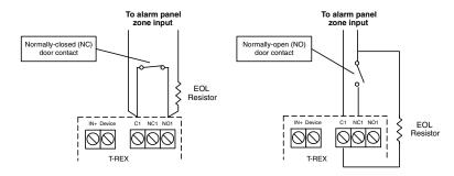
NOTE: The EOL resistor should be located within the T.Rex housing to provide proper supervision.
